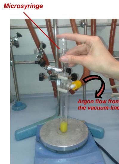
**Figure SM 7.7.1B** – Addition, under inert atmosphere, of the reagent.
