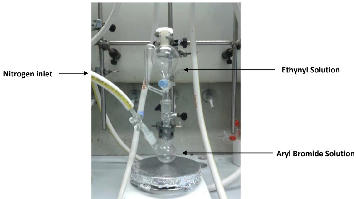
**Figure SM 7.4.1** – Typical experimental setup for the Sonogashira coupling reaction
