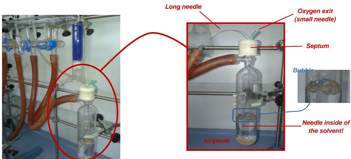
**Figure SM 7.7.2** – Deoxygenation solvent equipment.
