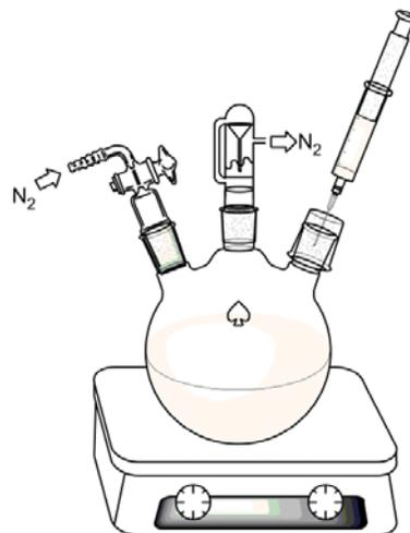
Figure SM 7.5.4: Setup for boronic acid synthesis
