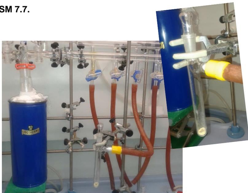
**Figure SM 7.7.1A** – Schlenk with solid reagents connected to the vacuum-line.
