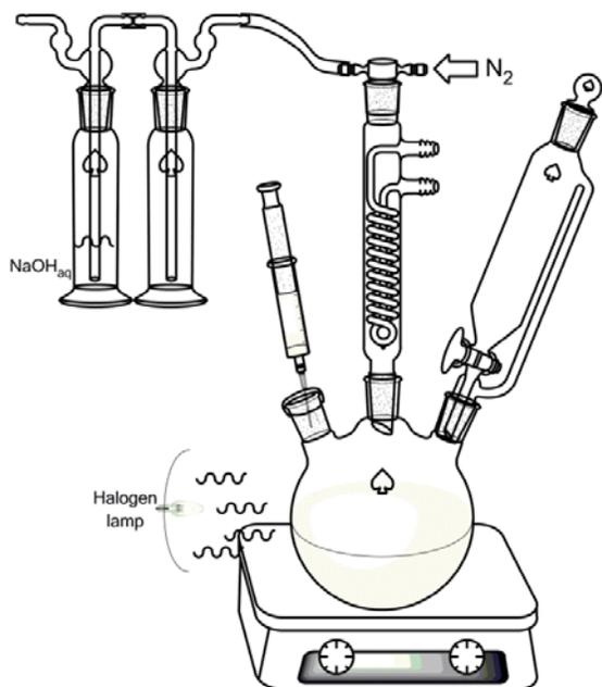
Figure SM 7.5.3: Setup for the bromination reaction
