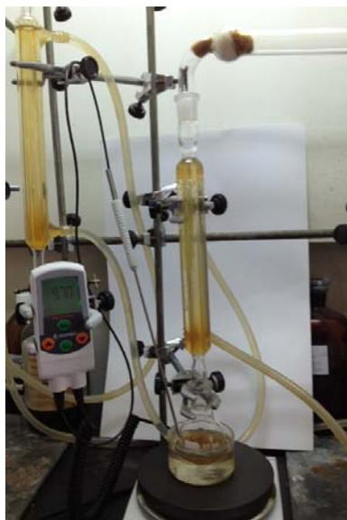
**Figure SM 7.9.2** - Synthesis of 3-vinyl coumarin (step2). Water condenser into the round-bottomed flask, equipped with a calcium chloride drying tube.
