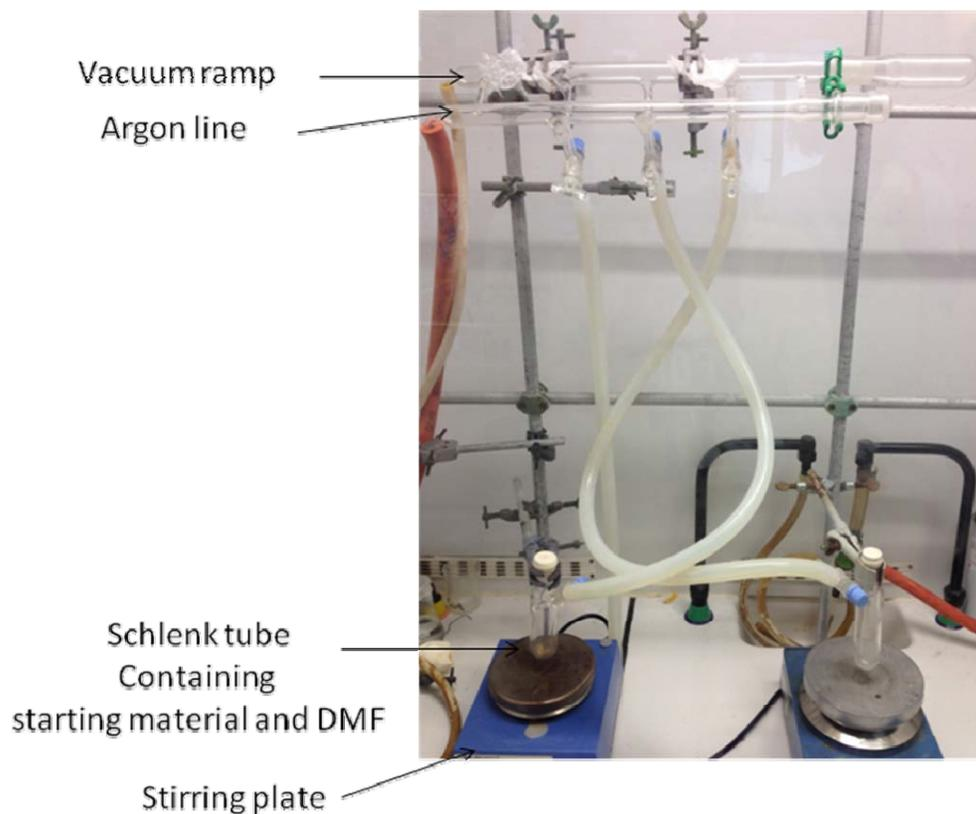
Figure SM 7.10.1: Preparation of the Schlenk tube
